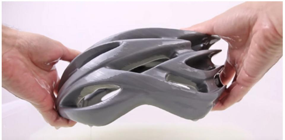
For most of the additive manufacturing technologies, it is required to post-process the printed parts in order to get them ready for use. However, in the case of FFF parts it is not always mandatory, and its main purpose would be to hide visible layer lines, to remove supports or to mitigate the anisotropic behaviour.
