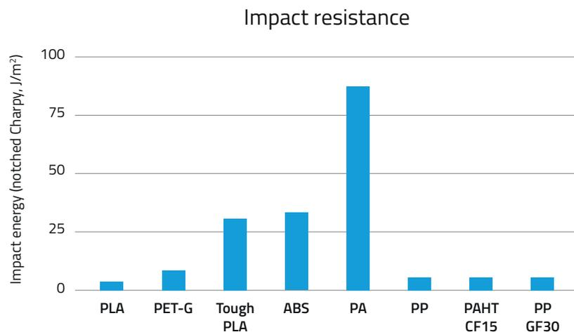
Graph 4: Impact resistance of BCN3D Filaments compared
