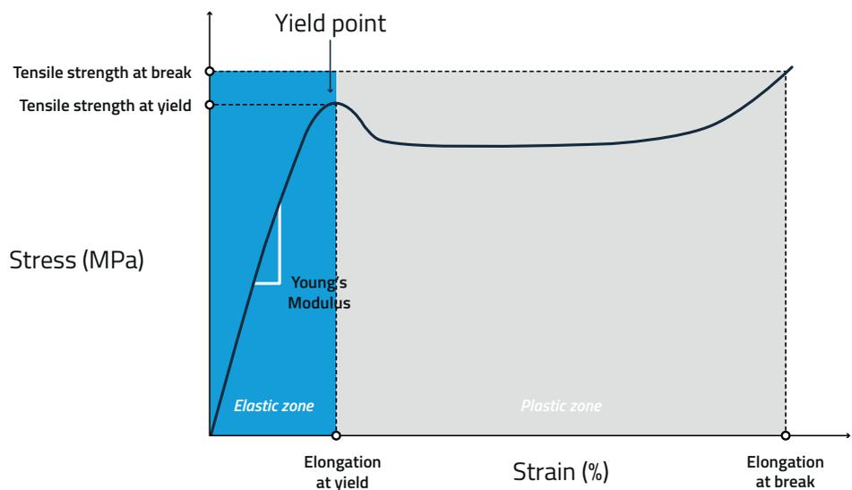
Figure 2: A typical stress vs. strain graph. BCN3D
