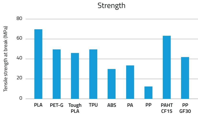
Graph 1: Ultimate tensile strength of BCN3D Filaments compared.
