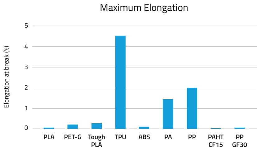
Graph 2: Elongation at break of BCN3D Filaments compared.
