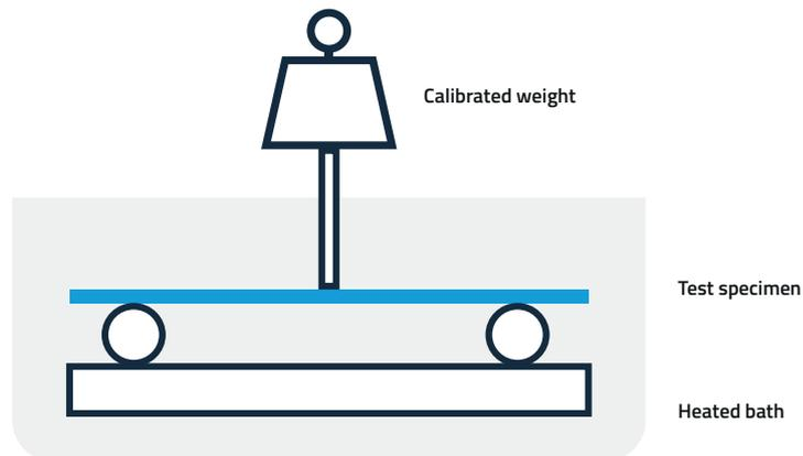
This loss of structural integrity generally happens close to the material  $T_g$ , which is the glass transition temperature. This is the temperature at which the polymeric matrix starts losing its rigidity, with the polymer chains uncoiling and gaining mobility. Above its  $T_g$ , a polymeric material behaves as a viscous liquid, and tends to occupy the shape of its container.
