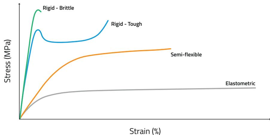
Figure 3: General tensile behaviour of different materials.
