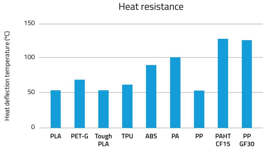
Graph 5: Heat deflection temperature (0.45 MPa) of BCN3D's filaments.
